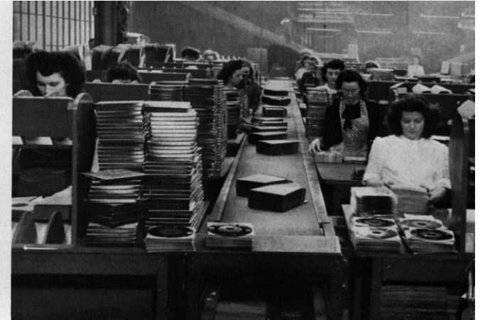
6 Here the finished records are placed in envelopes and then packed in containers for shipment to dealers and users.
