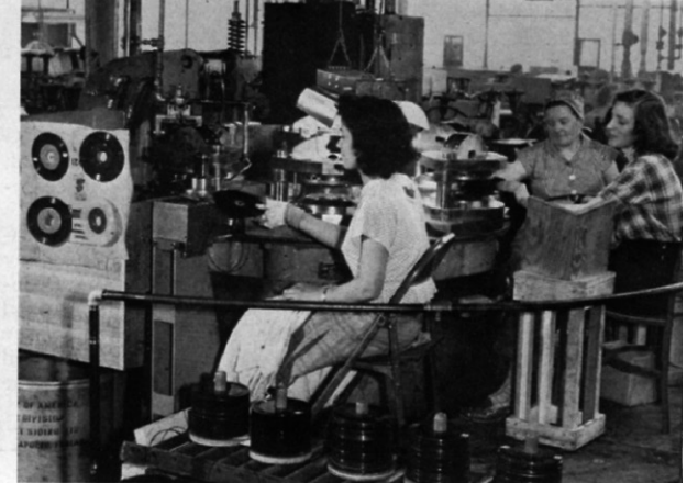
4 Each of these semi-automatic machines punches out the record's large center hole at the rate of 30 discs a minute.
