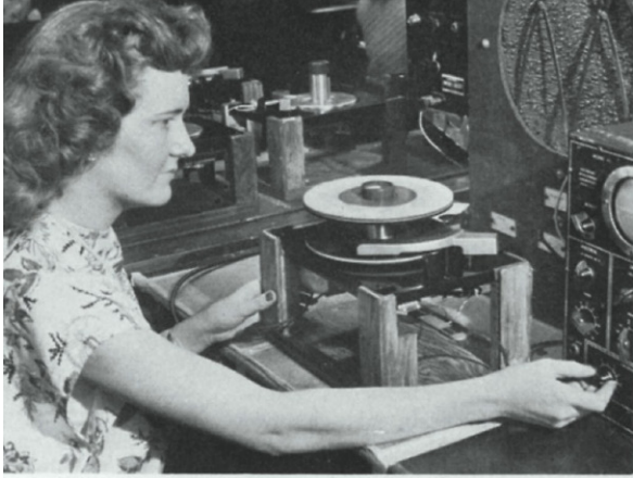
1 Maximum performance of the 45-rpm record player is assured by testing its operation with a sensitive oscilloscope.
