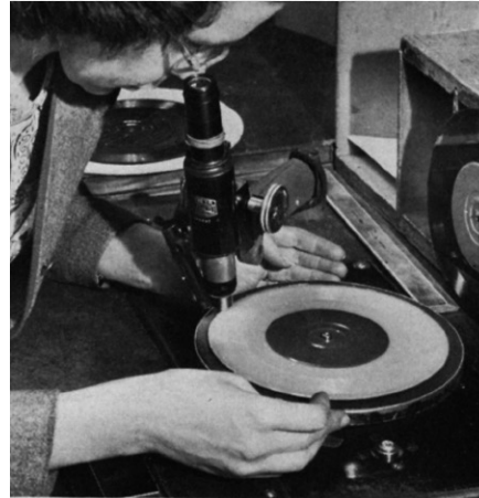
5 Exact centering of a 45-rpm record is assured by checking the movement of the outer rim under a microscope.
