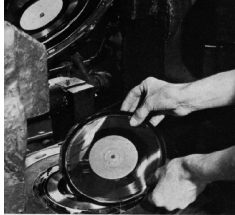
3 Excess plastic material, called "flash," is stripped from the outer rim of the recording following the pressing process.
